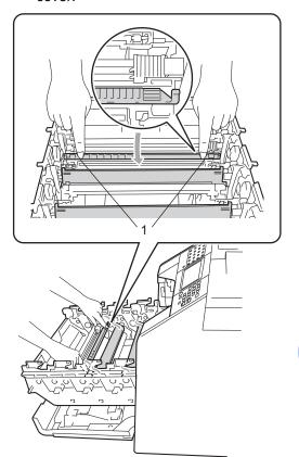
5 Clean the corona wires inside the drum unit by gently sliding the green tabs from left to right and right to left several times.
